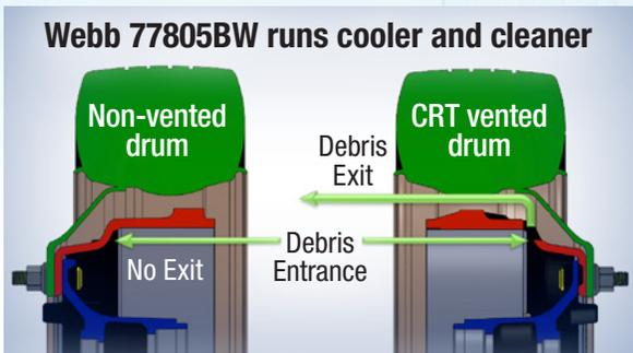
Webb Vortex with CRT™ vents provide a pathway for debris to exit the drum. This helps reduce grooving by minimizing the buildup of dirt, debris, and brake dust on the braking surface. Your brake system runs cooler, cleaner and lasts longer with Webb Vortex CRT.
